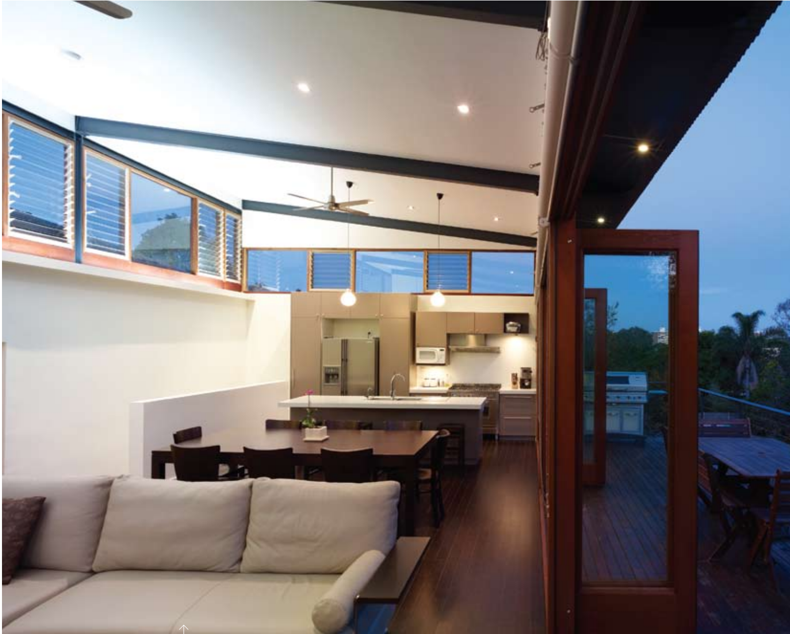
Louvred clerestory windows, bi-fold doors, high ceilings and reversible fans regulate the internal climate
